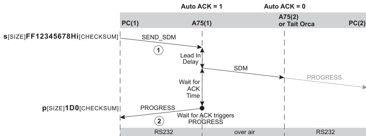
**SDM Auto ACK** is either enabled or disabled when the modem is configured. This is done in the A75 with the **PROGRAM** command or in the PGM programming software for the Tait Orca. If the A75 has SDM Auto ACK is set to '1' (enabled) in bit 7 of the [ITEM1] parameter of the PROGRAM command, then:
