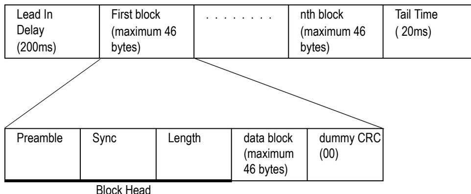
The default Transparent mode **Lead In Delay** is set to 200 ms. If a faster data rate is required the Lead In Delay can be reprogrammed to a minimum of 40 ms using the **PROGRAM** command. Note that if the Lead In Delay is set this low, Economy mode **must** be disabled.
