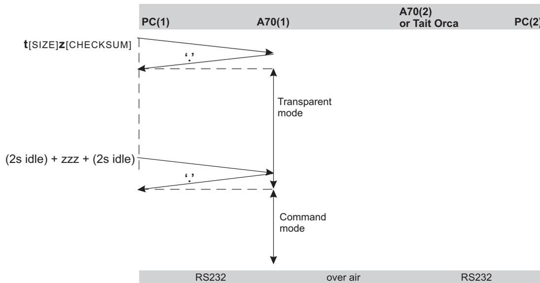
1. `t` is the message [IDENT] for a **TRANSPARENT** command telling the A75 to go into Transparent mode
