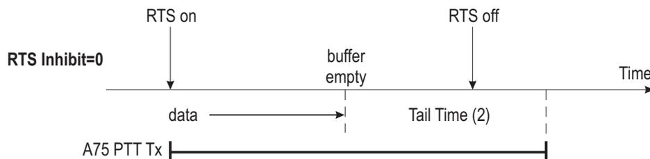
If the data stream has a gap, while RTS remains on, the A75 continues to transmit. This eliminates the data delay caused by the Lead In Delay at the start of each transmission.
