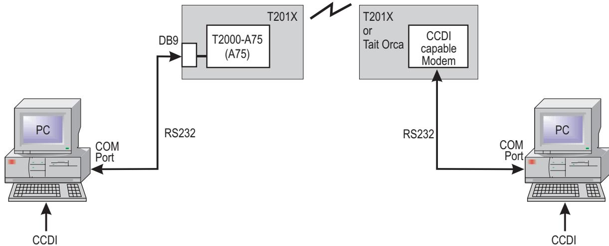
The A75 is fitted to a T201X radio and is connected to a personal computer (PC) by a serial line using five standard RS232 signals (TXD, RXD, CTS, RTS and GND).
