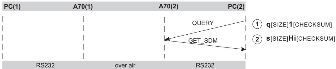
When it receives the SDM [QUERY](#) command, the A75 responds with a [GET\\_SDM](#) message (②). If there is no data in the EEPROM then the [GET\\_SDM](#) is returned with an empty [PARAMETERS] field.
