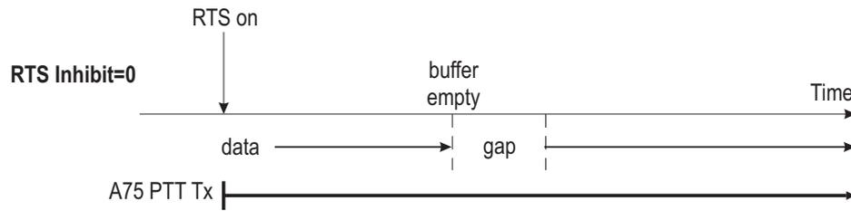
If a long data stream is sent, the A75 continues to transmit, but the T201X stops transmitting after the transmitter time-out. The transmitter time-out is set by the Transmit Time Duration which is set to a default of 60 seconds in the T2000 PGM programming software.
