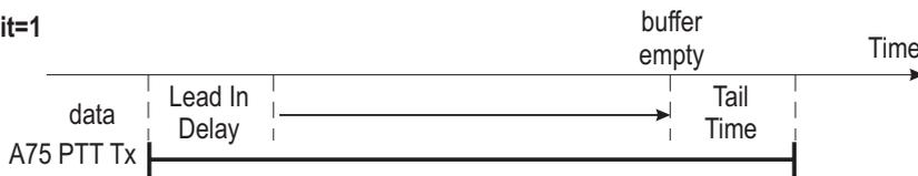
If 'Inhibit RTS Signal' is set to '0' (RTS not inhibited), when an RTS signal is detected (**RTS on**) the following sequences can occur depending on the structure of the data.
